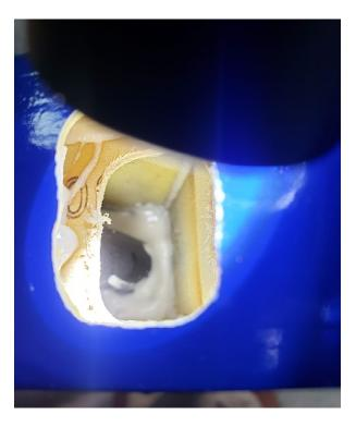
Stand wing vertical on trailing edge and use the long nozzle to apply glue to wing spar area between Rib #1 and #2.
