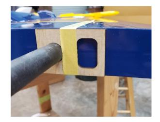
Use a Dremel tool with a Carbide Cutter to allow access to the internal structure of the wing.
