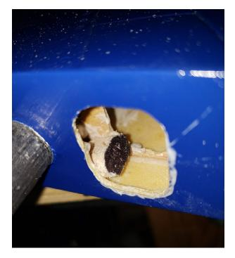
Using the extended nozzle, stand the wing on it's wing tip and apply glue around the spar and rib.
