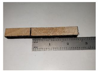
□ Use part of the end grain to make a plug .5" long to fit between the root and rib #1.
