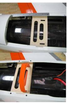
□ Test mount the 4S pack as shown. Notice the short piece of "fuzzy" adhesive backed Velcro on the battery. This restricts the fore/aft movement.
