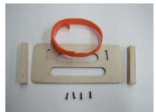
□ The plywood tray is set ¾" below the fuse flange by gluing the ¾" square balsa strips tangent to the outer edges of the plywood tray. Bevel the outside upper edges to allow fit into corners of the fuse flanges. A Perma-Grit scuff board is handy for this.
