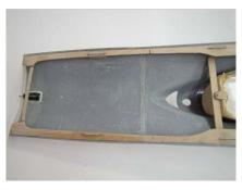
Bevel the aft tip of the EVF carbon fiber fairing that projects through the tailpipe so that it does not touch the 4S pack
