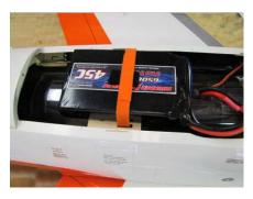
□ The two (2) 4S saddle cells are located full forward against the EVF mount. A Power Plug 3 connects the 3 packs in series to the EVF.
