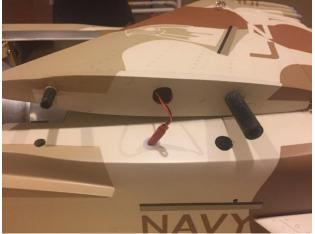
• Use a 9/64" driver to secure the clamp.
