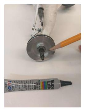
• Use a small amount of Axle Grease to the wheel axle. (BVM#5784)
