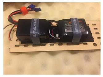
• Use (2) 12" battery extensions to connect the RX to the Lipo batteries.
