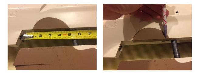
To help mark the Center of Gravity position when the wing is in place, you can use two Buttonhead screws on the bottom of fuse at the fuse wing joint. (BVM # 5625)
