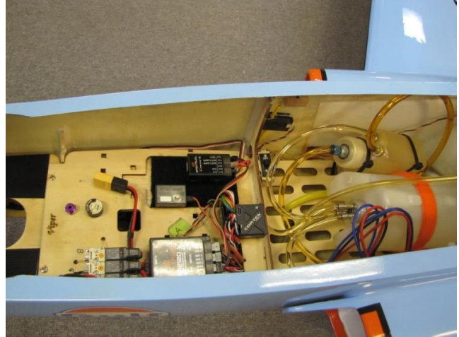
View of right side of mid forward fuse. See optional channel expander, flight logger, mini air pressure gauge, air fill valve, and Cortex Gyro.
