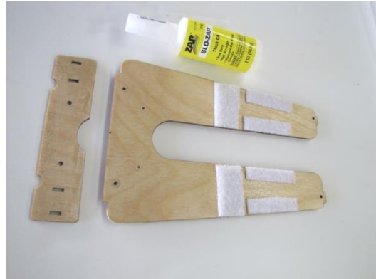
View of top side of tray and pump mount. A Zap or resin finish is applied for better adhesion of Velcro strips. Apply finish to both sides of the pump mount.
