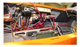
□ The receiver LiPo battery is mounted forward on the inlet duct. The switch is attached to the right side of the duct, both with adhesive back Velcro.
