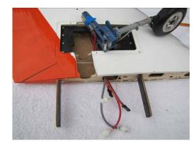
□ Retract unit is retained with (4) 4-40x1/2" flat head bolts
