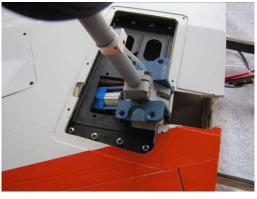
□ Plan to have the air tubing with disconnects and the flap and aileron servo wires exit the root rib as shown.
