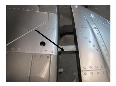
□ Secure each Stabilator using the 3mm bolts. A 2.5mm wrench will be used here.
