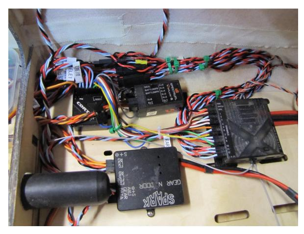
The demo model uses Electric Gear. We used the gear sequencer in the IX20 to close the main doors when the plane is on the ground. The stock Gear sequencer will only leave the doors open when the gear is down. We left the nose door plugged into the stock unit as it cannot close on the ground. The nose steering servo sits in the opening where the door would have to close.
