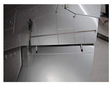
Picture for reference. The end of the metal tube has a bend in it. This will sit against the flap.
