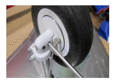
□ Lubricate the axles with Super Lube (BVM# 5784).
