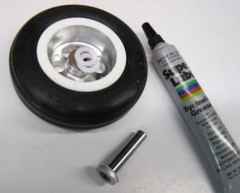
Reassemble everything, making sure the clear brake tubing is on the aft side of strut. Securely tighten the axle retaining bolt with a 2.5mm Hex Wrench.
