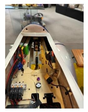
This is an Overview of our layout looking back and forward. If your plane came with a small plastic UAT mounted, BVM does not recommend the use of this tank. Use a actual BVM UAT as shown.
