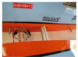
Make the (4) electrical connections. Note that they can only be plugged into the proper receptacles by physical design. Hand twist the Silver, Gold, and Blue threaded couples together. Turn only the ends that can swivel to avoid kinking the tubing on the female end.
