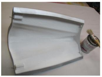
To reduce any effect of residual heat after engine shut down, apply 2 coats of BVM Heatshield (BVM#1940) to the inside surface of the engine
