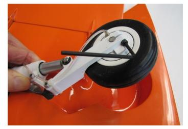
A variable speed electric drill with a Phillips head driver is handy to remove and reinstall the (6) screws that hold the retract unit in place.
