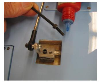
Remove the 2 set screws in each elevator, apply a drop of Z-42 then insert and tighten in both elevators. If you over tighten these it will warp the top skin.
