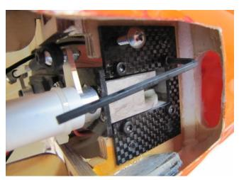
To remove the nose gear first remove the (4) socket head bolts. Use a 2.5mm hex wrench. Then remove the (4) Phillips head wood screws.
