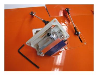
You can use a 2.0mm hex wrench to check the security of the nylon/aluminum ball/socket linkages.
