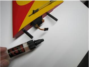
☐ Use BVM Dry Lube (BVM# 1947) on the Carbon Rods to allow easier installation into the wing and tail receptacles.
