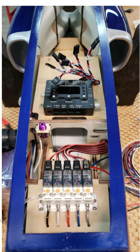
Gray- Brake Blue- Gear Up Red- Gear Down White- Door Open Black-Door Close
