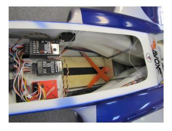
You can install the Receivers ON/OFF switch in the provided mount and install it in a location like the one shown here.
