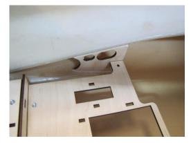
Build the Forward Battery tray as shown in the picture. Do not leave out the two small ply doughnuts.
