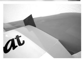
With booms fitted to fuse, install the alum bushings on outside of fins. Test fit with #6-32x1-3/4" phillips head bolts. Remove, then apply a drop of 5 min epoxy to bushings and insert them into the fin.
