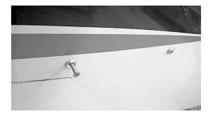
□ Cut opening on **inside** of fin for servo leads as marked may have been done at BVM.
