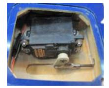
For flaps "up" servo arm is about 45<sup>o</sup>forward.
