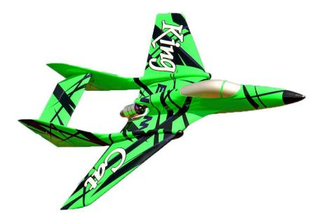
Length: 94", Wing Span: 80" Fuel Capacity: 4.8 Liters For 120 to 180 N Turbine
