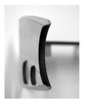
Before glueing in the UAT tray. Bevel the outside edges about 45 deg of the two vertical pieces.
