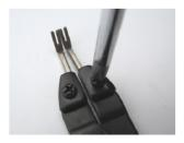
Securely tighten the screws.
