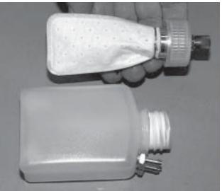
This shows the proper orientation of the sack in the tank. It is best to not open the tank unnecessarily so as to not disturb this setting. Note the teflon seal on the bottle cap threads.
