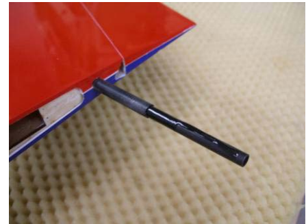
Photo 57 Epoxy applied to the steel tube
