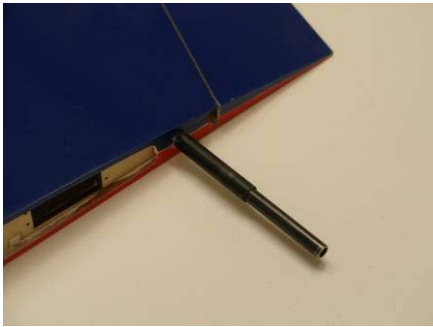
Photo 55 Steel tube into the CF spar
