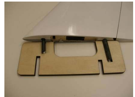
Photo 60 Test fit the front pin using alignment fixture
