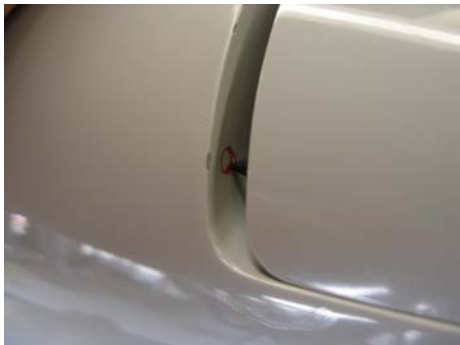
Photo 84 marking the hatch pin receptacles
