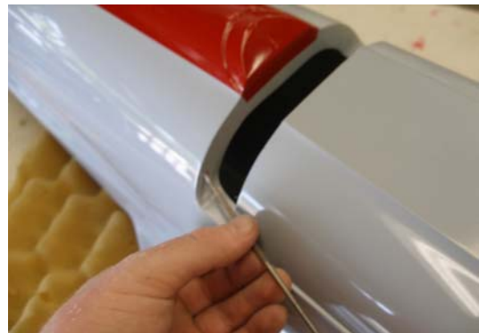
Photo 85 adjusting the engine hatch pin receptacles
