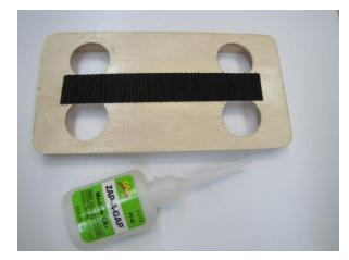
☐ Use ZAP RT to glue this battery tray to the fuse floor.
