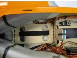
☐ The receiver/servo power battery can be retained in a piece of Jet-Foam shaped by you.
