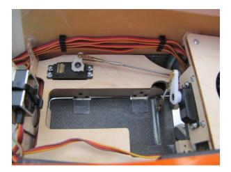
Forward equipment tray with radio switch and electric retract controller mounted for easy access.
