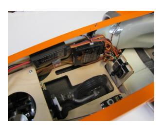
□ View of organized wires routed along left side of fuse next to nose gear steering servo. Linkage for nose gear door is also detailed here.
