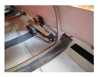
BVM "O" Clips are handy to bundle wires in fuse bottom.
