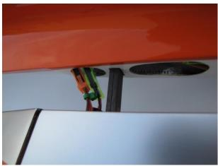
Electric retract and door wires connect at forward wing/fuse openings. EBrake connectors link up here as well.
