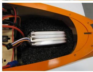
Apply another rectangular block of Jet-Foam on top of the battery and trap the ends under the fuse flanges.
