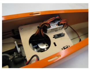
The BVM EBrake is located as shown. It is retained with 2 small button head screws through fuse bottom into the plywood side frame.
