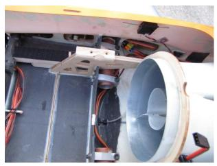
Wing Flap and Aileron servo extension wires connect at rear of wing / fuse junction.
