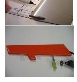
Use the same techniques to make the slots in the fin. Extend fin slots 3/8" towards the tip to allow for the swept hinge line.
