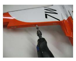
Use a tapered cone tool and 3/32" drill bit to allow injecting Aeropoxy.
