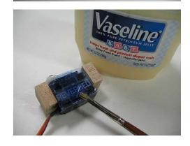
After sufficient test fitting, apply Aeropoxy to the maple blocks and a bit to the inside fin skin and carefully insert into the fin pocket. Use masking tape to hold in position until glue sets.
