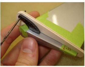
Use the template to check proper position of the control horn.
