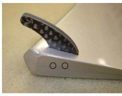
Use the control horn to set the depth of the slot. Trim the tab if necessary to avoid damage to opposite skin. Drill small holes in base of rudder to allow glue rivets to form.
