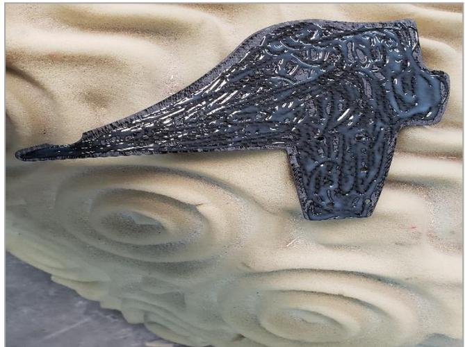
Once above steps are complete we are ready to start gluing. Start with the back side of the former and apply a bead of V-Poxy to the bottom of the former joint. Wipe this area to create a fillet.
