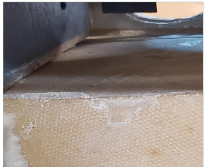
This is after the V-Poxy fillet is applied to the back of the former
