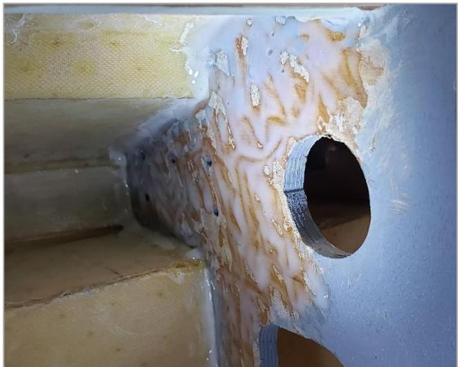
CF doubler in place and curing. The wing bracket bolts are what aligns the CF doubler to the former. This process is done in one shot. The outer edges of the doubler are held firmly to the former with small clamps until cured.
