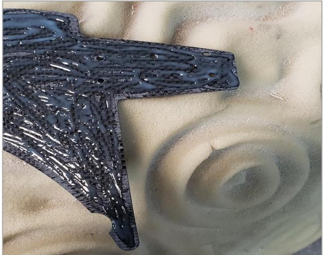
Apply V-Poxy to the former as well. At this time you are ready to reassemble the bracket on to the former. Use the bolts that came with the CF doubler as they are 2mm longer than the originals.
