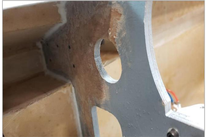
Sand the edges and backside of the CF doubler with 80 grit sandpaper. Make sure to clean the CF part before gluing.
