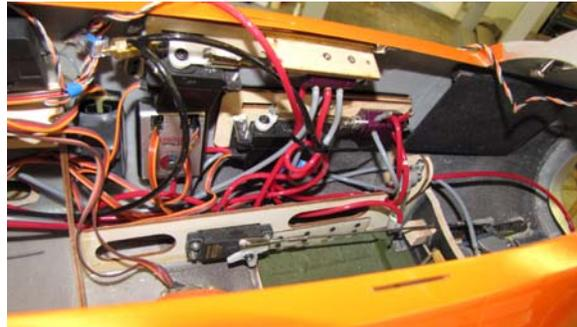
□ The JR Spectrum primary receiver is mounted similarly on the fuse side. Notice a remote receiver mounted to fuse bottom skin. Adhesive backed Velcro is used.
