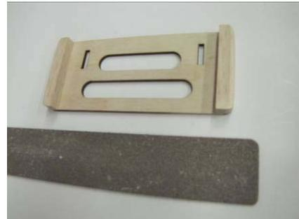
The front edge of the tray (note Velcro strap slots) is  $5 \frac{3}{4}$ " forward of the canopy hatch aft flange. Glue the balsa spacers (with ply plate) to the underside of the flange. Slow Zap works here.
