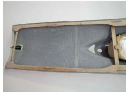
Be certain that the Hatch Latch is securely Aeropoxy glued to the hatch.
