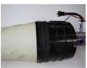
You can use a pencil or a wood dowel to spin the rotor to check for rubbing.
