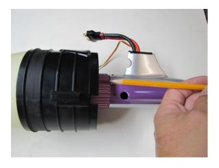
If the spinner is rubbing on the spike, you can use a sanding block to remove the flange on the back of the spike.
