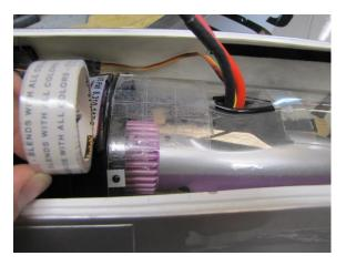
Once the pipe is in you can trim the pipe to match the rear opening of the fuselage. You can also remove the pipe and use flat black testers to paint the pipe on the outside.
