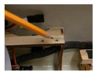
We recommend using some Qt poxy to hold the blind nuts in place. BVM # 9580.
