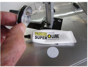
Apply Super Axle Lube BVM # 5784 to the axle from inside and outside access. Note the nylon spacer.
