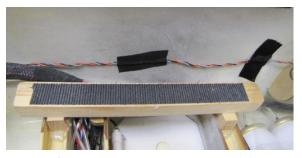
□ A strip of Velcro on the side of the fuse and the top of the battery rail is all that is required. Apply a C.A. or epoxy finish to the tops of the wood rails to improve Velcro adhesion.
