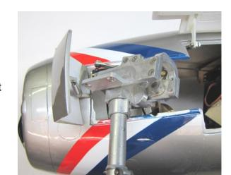
☐ Maneuver the retract unit to get it out of the model. Use a BVM Collar Tool to disconnect the pneumatic lines from the nipples on the cylinder.
