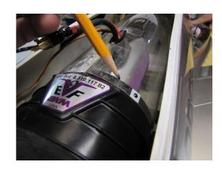
Use the 3M tape to seal the front opening of the tailpipe. Use one piece on the forward seam of the opening and then three pieces across the opening. This is a time-tested method that works.
