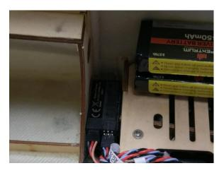
This example on a BVM plane used a regular Spektrum 9030 Rx and an X-plus expander. You can find the Rx channel mapping under Connecting Rx wires later in this manual.
