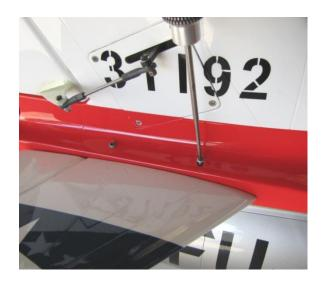
**NOTE**: The elevator neutral position is located at this point.
