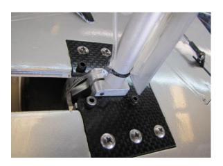
☐ Use a 1.5mm hex wrench to loosen the set screw that retains the axle. Check to see if there is a flat spot ground in the axle. If not, use a Dremel cutting disc to make one as shown. A matching cutter mark on the end of the axle helps to properly orient it.
