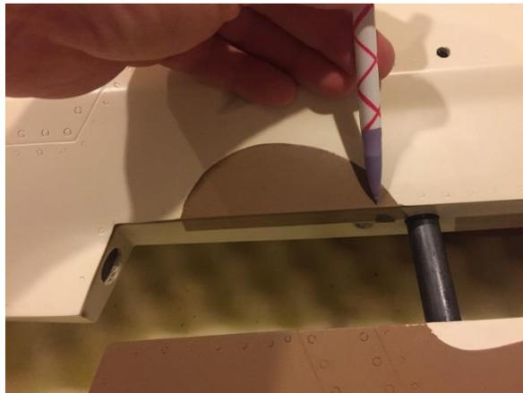
To help mark the Center of Gravity position when the wing is in place, you can use two Buttonhead screws on the bottom of fuse at the fuse wing joint. (BVM # 5625)
