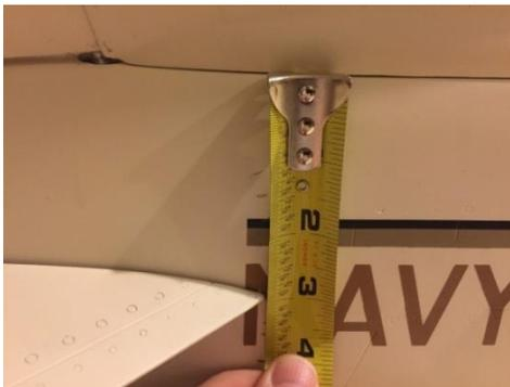
The Neutral point of the stab is 3" below vertical fin junction at the L.E.
