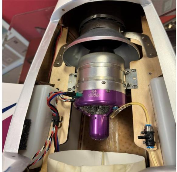
This shows the correct orientation of the electrical and fuel-in lines. As well as the fuel shutoff valve.
