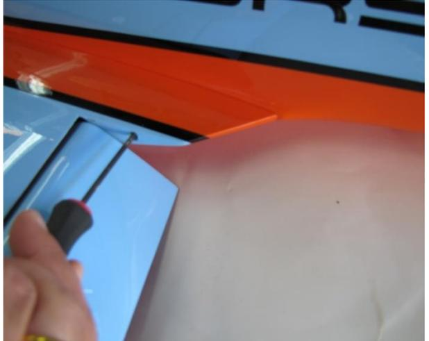
**FLAPS** - A plywood Flap Gauge is provided. Position it on top of the wing adjacent to the fuse joint.
