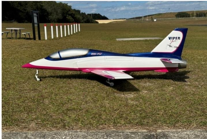
Length: 74" (1880mm), Wing Span: 73.7" (1872mm)
