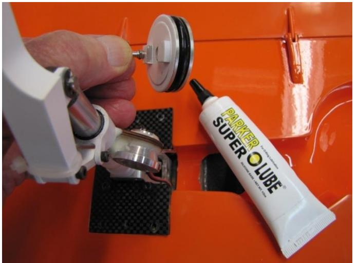
NOTE: To connect threaded air fitting at wing fuse joint - rotate the female fittings only - (Gold/Blue/Silver) to avoid a kink inside wing.
