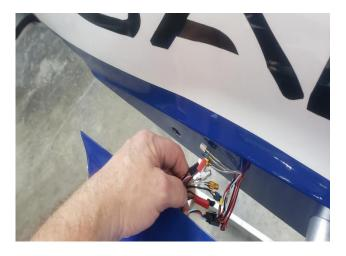
The wings are held by a front and rear receptacle. A 9/64<sup>th</sup> driver is all you need to secure the wings.
