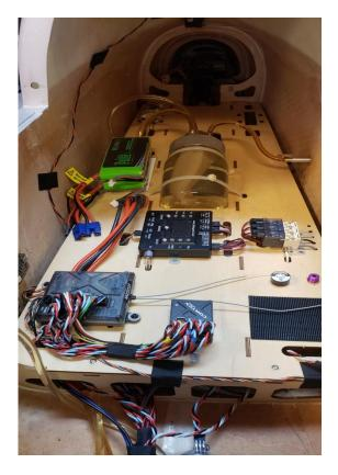
The BVM demo Renegade uses the stock UAT the plane is shipped with. If you decide to use the supplied UAT you must hold the UAT vertical and shake the tank during the first run up to ensure all the air is out of the Filter bag inside the tank.
