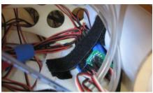
The "GEAR" wire coming from the main controller goes to your Receivers gear channel. The "LED" wire coming from the main controller goes to your Receivers channel of your choice, this will be the channel to control your lights The "LED" channel coming from the RX has three positions, Off, NAV Only, and NAV and Landing lights.
