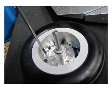
□ Lubricate the O'Rings with Super O-Lube (BVM# 5779).
