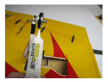
Lubricate the axles with Super Lube (BVM# 5784).
