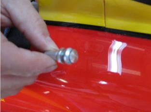
BVM used a small piece of fuel line to attach the fuel filler plug to the Fuel can.
