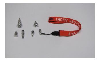
Install the fittings to your overflow/taxi tank. Use an overflow tank while fueling to prevent spillage and to ensure fuel tanks are full before flight.
