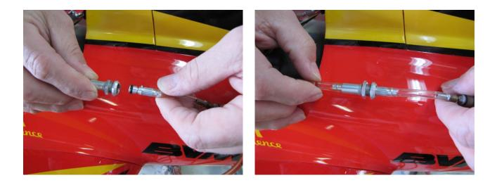
After removing the filler plug, insert the stop plug to help maintain the seal.
