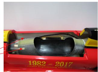
□ Remove the (2) M3x8 SHCS inside the bypass.
