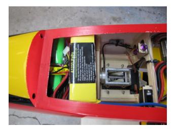
The batteries will mount in the nose of the Bandit EVO as shown on the battery tray.
