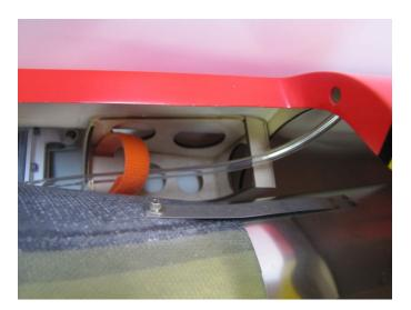
Install A BVM UAT in the mount provided, located along the right rear fuse side in the engine hatch.
