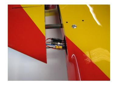
Secure each wing by tightening the (4) clamp bolts with a 9/64 ball wrench.
