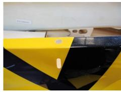
☐ Glue the Hatch Latch using QTpoxy.
