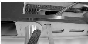
□ Measure the distance from inboard edge of F/G flange at the wing root to the center of the bolt hole. Apply a piece of masking tape to wing bottom centered on the slot and drill a small pilot hole.
