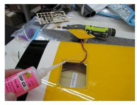
☐ Scuff both bottom sides of the elevator control horns to aid in adhesion.
