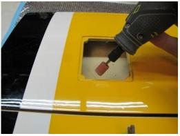
□ Using the servo plate, drill the four corner screw holes with a 1/16 bit, then reinforce the holes with a drop of thin CA.
