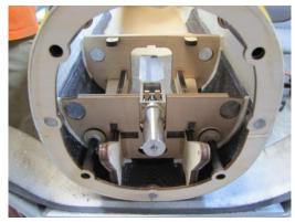
With the Nose Cone taped in place, Glue the two upper tube supports in place with Vpoxy or Aeropoxy.
