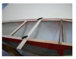
☐ After all canopy hooks are installed; apply Aero or Vpoxy to each hook and the ply frame.
