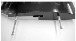
□ It is necessary to drill 1/16" vent holes in the fore and aft arrow shafts in the stab. Drill through one wall only of shafts. This allows air to escape when alum inserts are glued in. Sight through shaft, if open, one hole is sufficient, if plugged in the middle drill two holes, one each per servo pocket. Use a 6" long 1/16" bit. Protect stab skin while working
