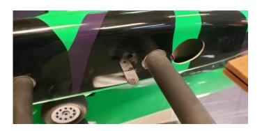
Make ink marks vertical and tangent to tubes as shown. Make 1/4" holes as shown to allow injection of Aeropoxy later. Reach through adjacent opening in boom sides and apply a bit of 5 min epoxy to short carbon tubes and boom sides.
