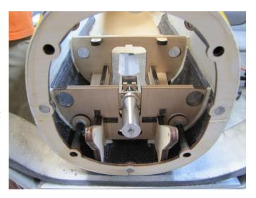
Note: It is a good idea to bevel the edges of the formers where they meet the fuse to allow for better glue adhesion Also finger wipe to create a fillet with the glue for a cleaner install..
