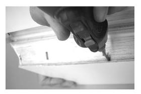
□ Use a 3/32" carbide cutter to cut slot for horn as marked. Slot must be parallel to and align with top flap skin. Test fit horn into slot. It should be fully seated against flap L.E.
