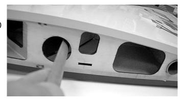
☐ Chamfer inside edge of 1.26" carbon tube with a drum sander to ease entry onto aluminum tube
