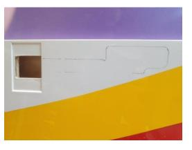
☐ Test fit the retract. May have to expand parts of the opening. Mark the center of the four screw points for the flexplate. Drill down about .6" with a 3/32 bit. Secure with four M3.5x16 screws per retract.
