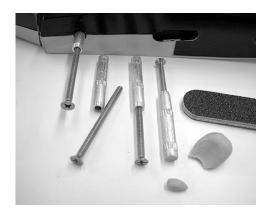
Proper depth of insert into stab leaves approx. 1/2" of insert exposed. Just covering 2nd row of knurling. Tapered end allows easy insertion into fin. Note opening for servo leads, match to that in fin.
