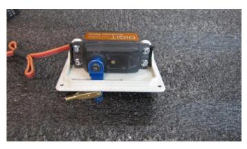
☐ Scuff sides of rudder control horns (marked "R"). Follow same procedure as described for elevators to install horns with Aeropoxy
