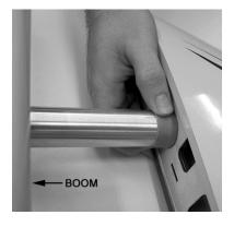
The inboard end of the flaps will need to be trimmed to clear the boom. Cut out the u shaped scribed piece of the flap end and also remove the mold flashing.
