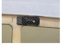
☐ Taper the forward end of the carbon fiber receptacle and glue into place lining up the holes.
