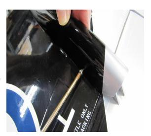
This is the small trailing cover for the Aileron Linkage. Using tape and a pencil mark the location of the cover. Then cut out the area where you will apply the glue.
