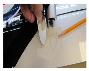
Use a small drill bit to make some anchor holes in the Aileron as well as the cover itself. Using QT-Poxy secure the cover to the Aileron.
