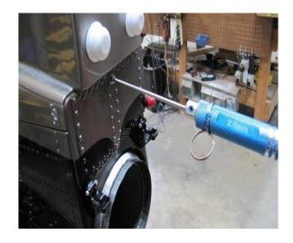
After the Top Cap is removed you will access to the Mounting Brackets. There are 4 bolts, 2 on each side that hold the Bracket in place. Remove one at a time and apply Z-42 Loctite to each bolt and re assemble. You will need a 3mm wrench to complete this step. .
