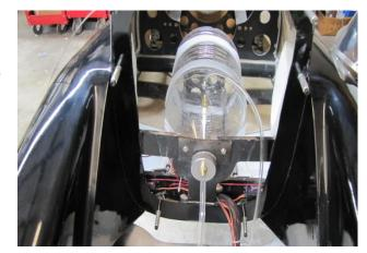
Once the 2 halves are together repeat the same process as you did for installing the pins into the rear half. A small drop of Z-42 will secure the bolts into the pins. Then install the 2 front duct screws. use a small amount of Z-42 on these as well.
