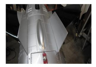
The Ventral fins are secured by 3 self tapping screws per side.
