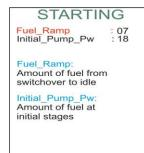
There are only two adjustable parameters in this sub-menu, "Fuel Ramp" values and "Initial Pump Pw".
