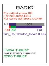
**Note:** For FUTABA systems you must reverse the throttle channel, Jeti and JR systems require non-reversed settings, other systems will require verification using the graphical display in the Radio Menu.
