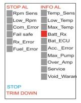
"Temp\_Sens" indicates a temperature probe failure.
