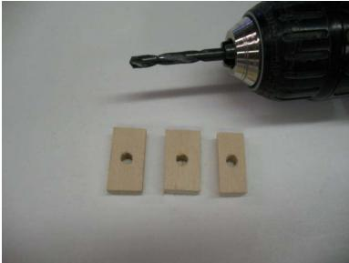
□ Use a Perma-Grit large square file to make the 3/16" holes square to accept the hinge stem. Hand fit a basswood block to each hinge stem until it is snug, yet stands
