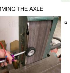
Remove the excess axle protruding from the lower strut assembly. It is not necessary to make this flush; just enough to prevent interference with optional gear doors or extend beyond the wing's lower skin.
