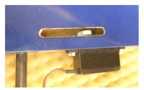
Cut the slot for the servo arm as marked on the bottom skin. Adjust for proper clearance once the servo is installed and linkage connected.
