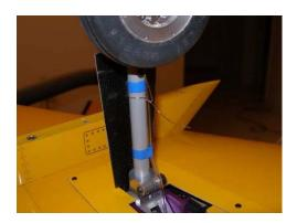
Use safety wire to attach the CF strut door attach block to the strut.
