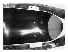
The aft 3-4 inches of the bypass is treated with 3 brushedon coats of BVM's heat shield (#1940). Two 4-40 x ½" SHCS with washers hold the bypass to CF angle brackets mounted to F-5.
