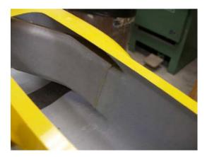
Apply additional SLO-ZAP to help secure the inlet to fuselage joint. Allow the glue to run around the inlet.
