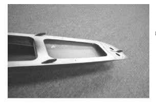
□ Install the (4) molded side canopy hooks into the canopy hatch frame one at a time.
