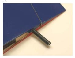
NOTE: There have been a few occurrences of the gauling of the Carbon Fiber tube in the aluminum stab mount. The problem occurs if the setscrew (in the aluminum stab mount bracket) is not backed out sufficiently, or there is a raised burr around the setscrew-threaded hole.
