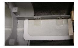
Begin by screwing the nylon hinges to the plywood nose gear door hinge mount.
