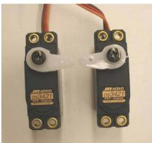
Use the JR Matchmaker to orient the servo arms to be slightly forward from perpendicular. Install the grommets and eyelets from the top of the servo as shown.
