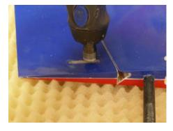
Use a Perma-Grit flat file to adjust and fine-tune the control horn slot.
