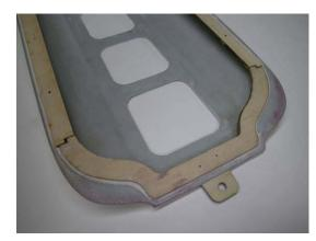
NOTE: Early kits will need the front and rear former of the engine hatch relieved to clear the engine by-pass as shown.
