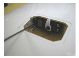
After routing the aileron servo lead to the flap servo pocket, install the four #2 servo screws. Use a high quality ball driver to avoid stripping the head of the screws. A small notch can be made in the servo cover flange to allow more motion if an "L" wrench is used.
