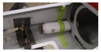
Below are a series of photos that can be used for ideas to route air lines. On our first prototype, BVM used additional air quick disconnects to allow the ECU tray to be removed quickly and easily without cutting airlines.
