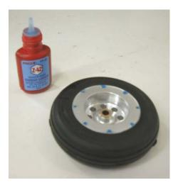
Before tightening the tire screws, apply a drop of blue Thread Locker to the threaded holes. This prevents the screws from backing out under the vibrations of braking. Carefully tighten the screws, avoid stripping the threads.
