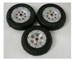
Use the supplied drill bit in a drill press or Dremel tool to drill the through holes for the tire mounting screws. Start from the smaller, threaded side and drill through to the larger hole on the opposite side of the rim.
