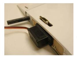
Install the servo with the servo arm as shown, once in place rotate the arm through the stabilizer skin.
