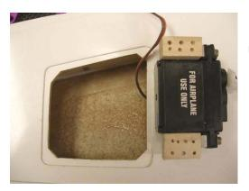
Apply SLO-ZAP to the maple servo mounting blocks and hold the servo in place until the glue has cured.
