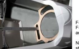
F-6 is a mushroom shaped 1/8" ply former. It is installed 6" aft of F-5 (the rear wing mount former). Sand the edges for a relaxed fit and glue it in place with AeroPoxy.
