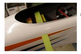
Use masking tape to pull the fuselage together to match the canopy hatch outline.
