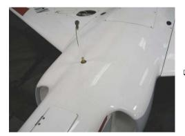
Add the fuel system vent in a convenient location on the bottom of the aircraft. Plumb the two vent lines from the main tanks through a "T" connected to the final vent fitting.
