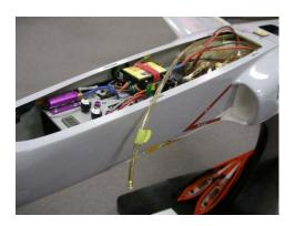
Plumb the two main tanks together with a "T" fitting connected to the vent of the 8 oz center hopper. The center hopper feeds the UAT through one of the brass fittings. The second brass fitting is for the refueling line. The 6mm line from the blue aluminum fitting of the UAT goes to a 6mm to 4mm brass reducer and finally to the input of the fuel pump.
