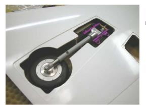
Temporarily fit and remove the landing gear assembly into the wing. It will be necessary to open the flanges around the retract unit and the wheel well a small amount to allow easy installation and removal. Use a Dremel sanding drum for this task.
