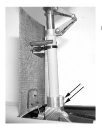
Attach the front door to the strut using the laser cut ply parts.
