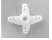
Use the long arm of the standard 4-way servo arm. This length is very important; the elevator linkage system has been designed to provide sufficient elevator surface travel and the required amount of power for 200 MPH flight. Using alternative servos or arms may unnecessarily risk the plane.
