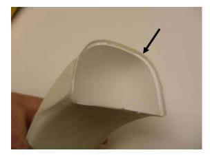
Remove 1/4" of the seam joint on the top and bottom of both inlets as shown. This allows the inlet extension to slip over the inlets. Make sure to scuff all gluing surfaces in the fuselage and on the inlets.
