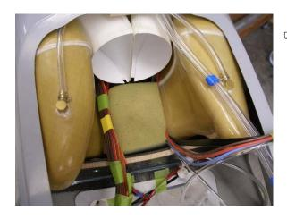
Secure the header tank with (2) #64 rubber bands.
