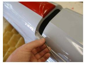
Drill these receptacle holes small, then use a Perma-Grit round file to adjust the size and location necessary to achieve a proper fit.
