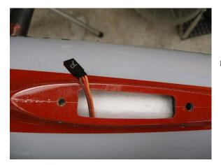
Install heat blanket over the elevator servos and under the rudder servo. Use aluminum tape to hold in position.
