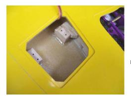
Remove the servo and use scrap balsa to reinforce the front maple block. Apply AeroPoxy to create fillets around the blocks.
