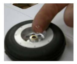
Apply a large drop of Super O Lube BVM #5779 to the brake drum surface of the wheel. Wipe this in until an even coat is distributed; apply an equal amount to both main wheels. At this time apply axle grease BVM #5784 to the wheel bushings and reinstall the wheels onto the struts as described earlier. Now the main wheels and brakes are complete.
