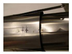
□ The distance between the inner pipe and the tail cone of the JetCat P-60 is 1.5"
