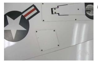
Position covers in place, masking tape can be helpful to hold the correct position. Use a 1/16" drill to make the pilot holes for the 3/8" button head screws.
