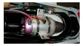
□ JetCat P-60 is mounted as shown. Note the position of the glow plug. Use a strap around the engine nozzle to lift it to center of the bypass while tightening the 6-32 screws in the metal straps.
