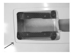
Install the flex plates into the wing using four 4-40 x ½" SHCS. It is necessary to remove a little of the F/G flange for clearance of the driver.
