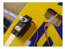
Helpful hint: A piece of yellow Nyrod makes a very good tool for pulling servo leads through composite structures. Simply bend the last (1) inch very slightly to allow a spinning action to help guide through formers and ribs. Use masking tape to temporarily attach the Nyrod to the servo connector, pull gently through the structure to avoid damage to the servo lead.
