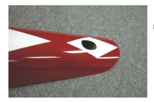
Enlarge the hole in the AFT end of the canopy hatch per marking. This allows access to the nylon bolt and a finger to properly engage the hatch to the fuselage.
