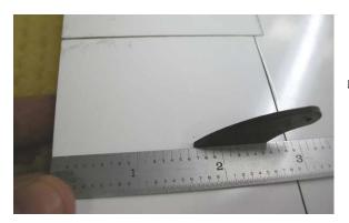
The trailing edge of the aileron horn is designed to be 1.7" from the trailing edge of the aileron. Make sure the horn flange sits flat on the skin surface.
