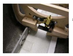
□ Trim the plastic arm as shown and orient the air fittings for the best possible routing as shown in the photo.
