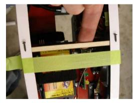
Drill the fiberglass flange and wood support stick with a 1/16" drill. Install the wood support using #2 x 3/8" button head screws.
