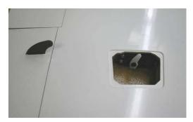
This is the completed aileron servo and control horn installation. Note that the servo arm is rotated forward one tooth, approximately 10 degrees.
