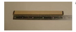
Trim the maple stick to approximately 5". Bevel the front corners to clear the glue fillet of F-1. The maple stick is glued to the rear of F-1 flush with the top edge.
