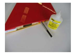
• Use a round Perma-Grit file to fine-tune the front hole to fit the anti-rotation pin.
