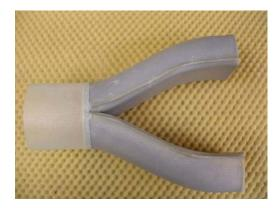
Trial fit the inlet extension over the inlets, some additional sanding on the circumference of the inlets may be needed; the extension should be a snug fit.
